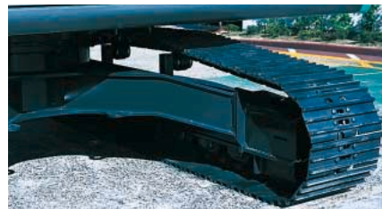
New design of crawler frame
